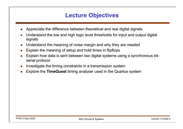
In this lecture, we will first examine practical digital signals. Then we will discuss the timing constraints in digital systems. The important concepts are related to **setup** and **hold times** of registers and how these, together with delay time of combinational circuit, determine how fast a digital system could run at.
